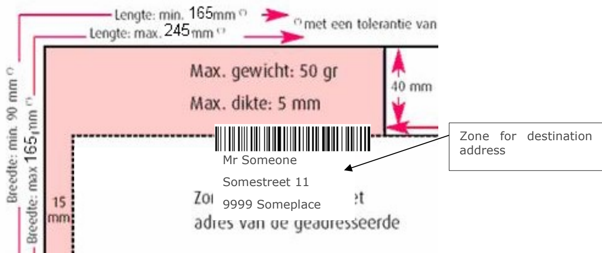
Figure 13: Placement of barcode
