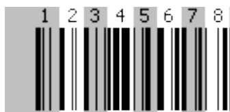
Figure 41: Code 128 Encoding Example
